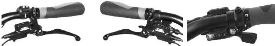
When braking hard by pulling the brake levers towards the handle bars, you should not push the braking force to its upper limit. Or, the braking distance will be extended and there is a risk of accident. Adjust the brake levers as mentioned above.
