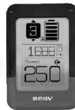
ON: Make sure that the battery is installed on the bike and the battery lock is switched to "ON (red)." The screen starts to display. Check that the system is on. The instrument enters the main page as shown, including assistance level, battery power, total distance and speed.
